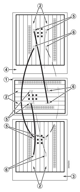
Figure 47. 3-way ICL cable connections between a SAN384B chassis and two SAN768B chassis.
